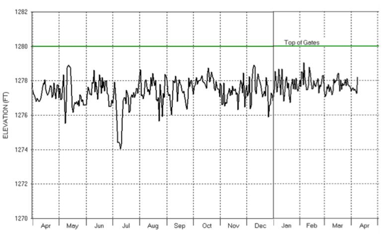
Apalachia has very limited storage in its normal 6-foot operating range (EL. 1272 to 1278) and it is primarily a run-of-the-river project.
